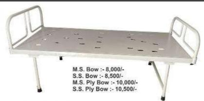
Made form 18 Swg. Uniformly perforated sheet mattress Bed frame made in 60 x 30mm Rect. ERW tube. Leggings made in 30mm X 30mm ERW Square tube Bows completely stainless steel 30mm Dia. Optionally available with S.S. Side Rails for patient safety, Stainless Steel head and foot and bows, telescopic. Adjustable I.V.Rod, 100 mm dia. Revolving castors. Pretreated & epoxy powder Coated Suppliedin KDC.
