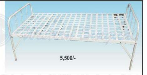
Made form 4mm Uniformly welded wiremesh with M.S. tubular head and foot end bows Bed frame made from 50 x 25xE.R.W tube with Leggings made from 30x30mm Square ERW tube Optionally available with S.S. Side Rails for patient safety, Stainless Steel head and foot and bows, telescopic. Adjustable I.V.Rod, 100 mm dia. Revolving castors. Pretreated & epoxy powder Coated Supplied in KDC.
